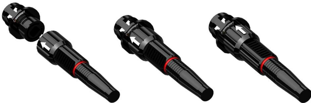
Fig. 7 The arrow part of the fiber connector is at the top, insert the fiber connector into the socket and then turn the arrow part clockwise.
